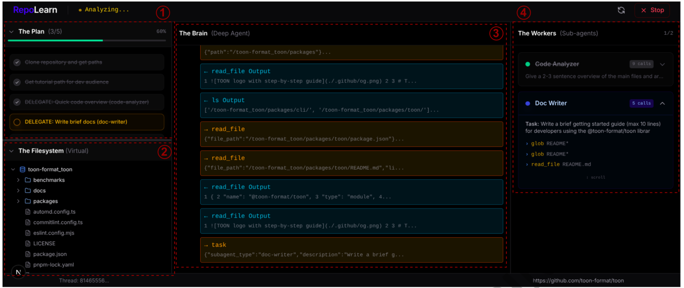
Figure 2: The 4D Observability Dashboard. (1) Temporal : The Planner Panel tracks the high-level TODO list. (2) Spatial : The Virtual Filesystem provides a real-time view of the agent’s environment. (3) Cognitive : The Brain Panel streams internal reasoning and action streams. (4) Hierarchical : The Worker Grid displays sub-agents executing scoped tasks with isolated context windows.
