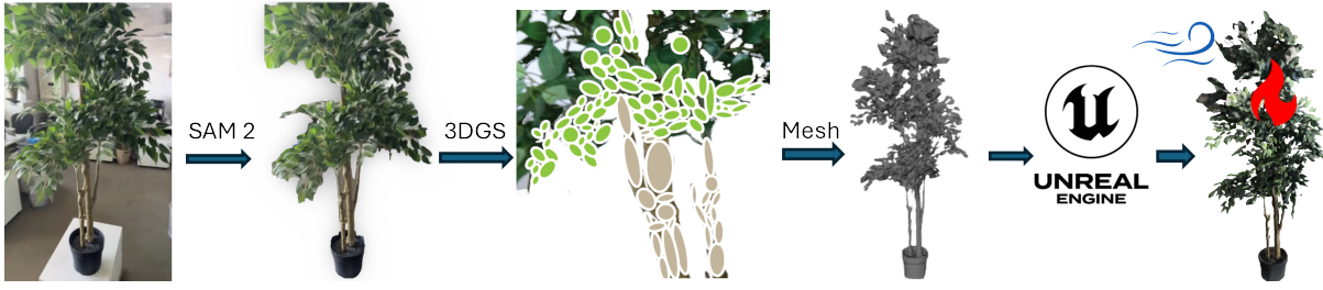
Figure 5: Pipeline of our 3DGS-based tree modelling.
