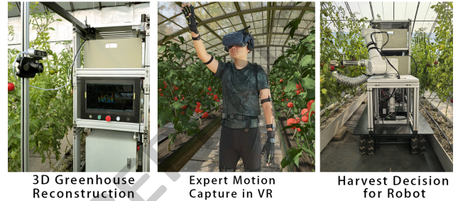
Figure 1: VR-guided harvesting: From 3D greenhouse reconstruction (left) to expert motion capture (middle) and robotic decision-making (right), offering new paradigm for data-driven algorithms.
