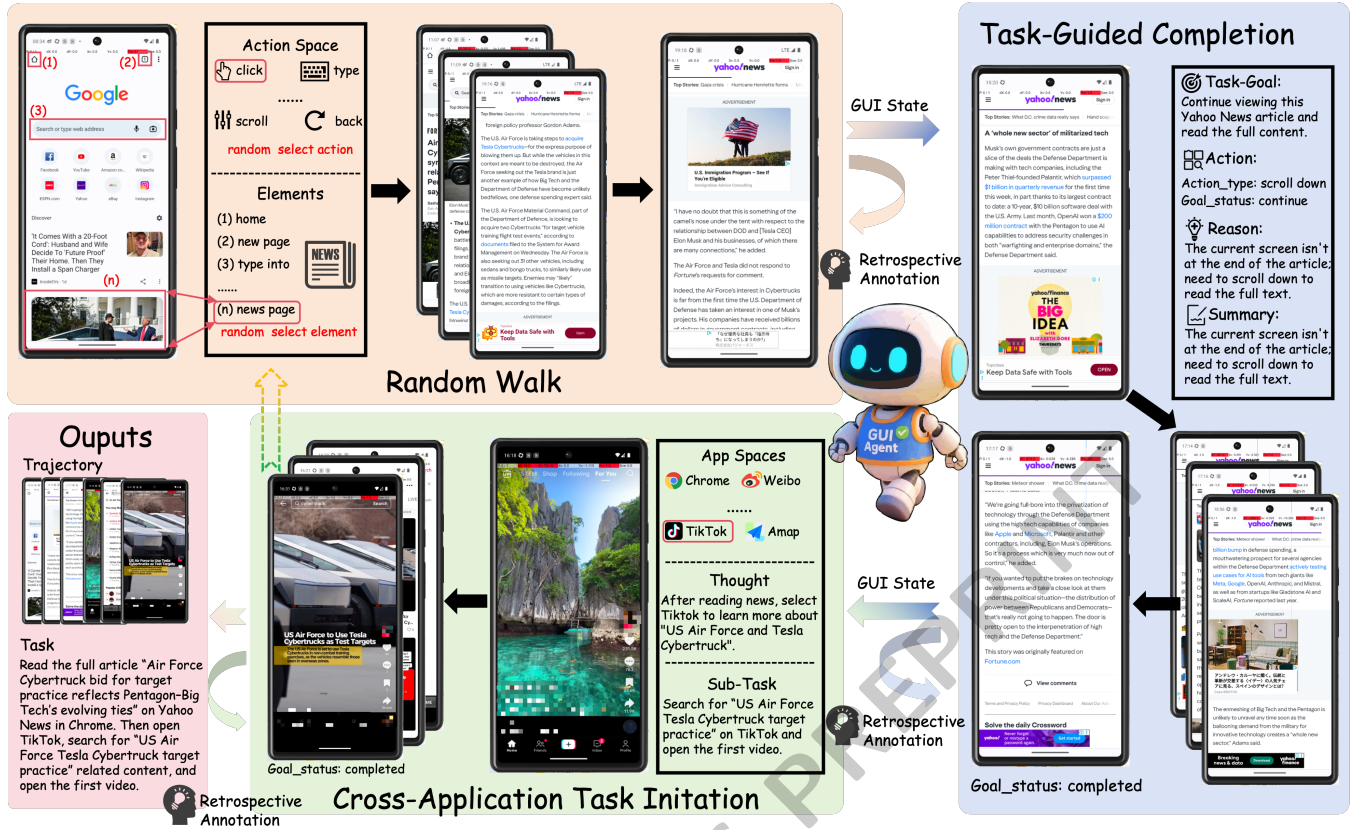
Figure 2: Overview of GUI-ReWalk Framework. Starting from a random app, GUI-ReWalk performs Random Walk by selecting actions and interacting with elements step by step; it then transitions to Task-Guided Completion to complete minimal-step tasks forming a stride, followed by Cross-Application Task Initiation to propose and execute new tasks in related apps. After each sub-stage, Retrospective Annotation records executed actions and GUI states. This cycle repeats across multiple strides to generate complete trajectories and overall task objectives.
