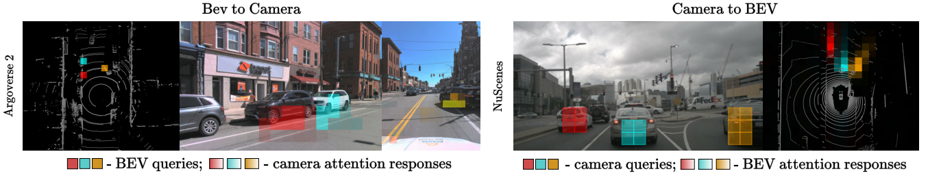
Figure 3. Cross-attention visualization demonstrating consistent correspondences between BEV queries and camera tokens. (Left) Image attention heatmaps for selected BEV queries, (Right) BEV attention heatmaps for selected image queries. These visualizations confirm that the implicit BEV projection learns geometrically correct camera-to-BEV transformations.
