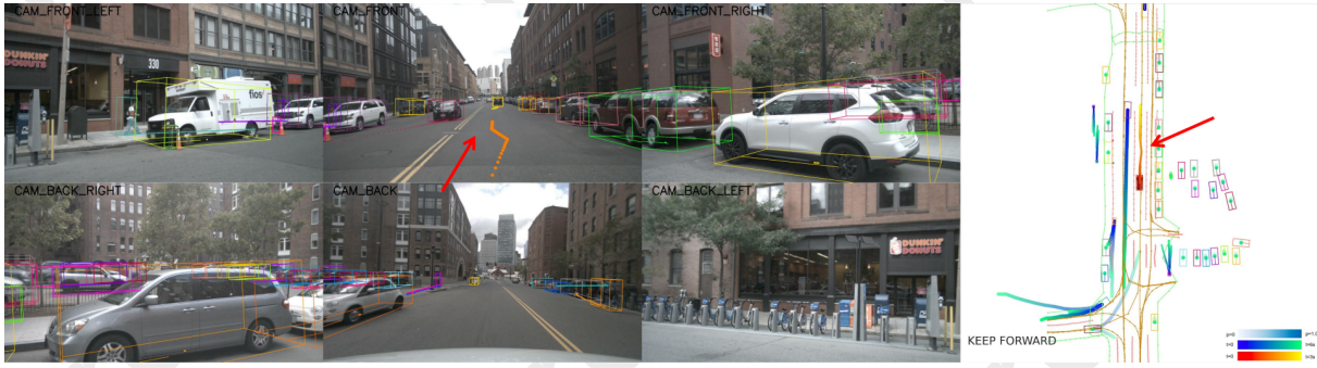
Figure 4: The qualitative visualization of the planning trajectories. The images from six cameras are shown on the left. The predicted trajectories of traffic agents and the planning result of the ego vehicle are shown on the right. The color intensities of these trajectories vary according to the probability p and the time t . The red arrows highlight the environments which most likely influence the ego vehicle planning.
