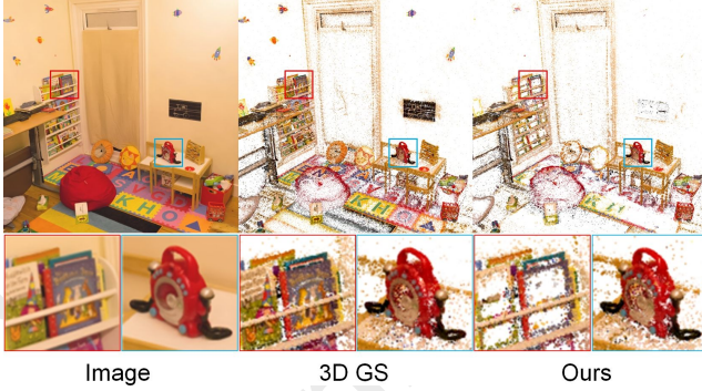
Figure 1: Visualization of Gaussian distributions and corresponding rendered images. The hybrid representation significantly reduces the number of Gaussians in texture-rich regions while maintaining Gaussian density in geometrically complex areas.
